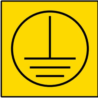
Warning: This equipment must be protectively earthed
