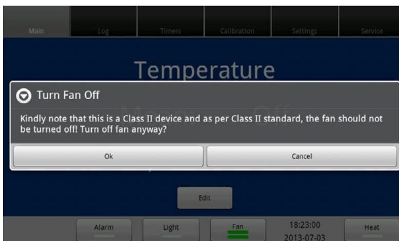
The fans of this unit are designed to run at all time. If you stop the fans, this warning appears.
