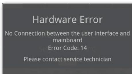
In case of a hardware error a message and an error code will be shown.
