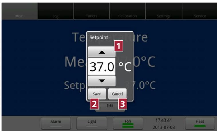
Press the arrow buttons **1** to adjust the temperature from 25 - 42°C.
