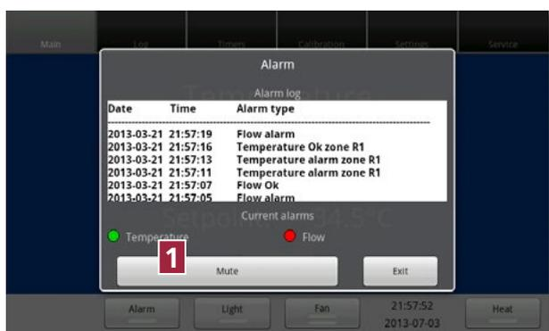
The alarm box shows information about the current alarm. Press **Mute 1** to turn off the audio alarm's sound.
