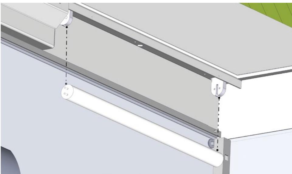
**3** Pull the tube gently down. Replacement is the reverse of removal.
