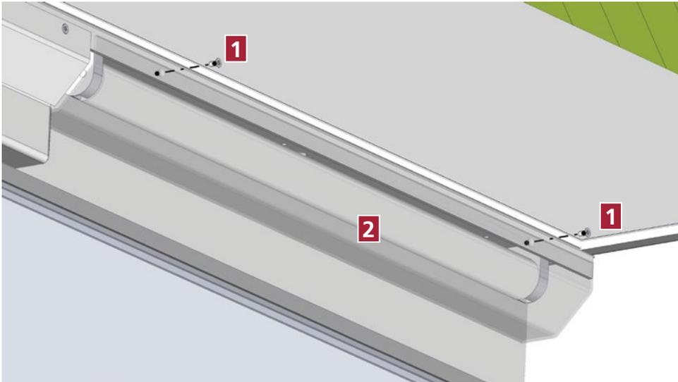
**1** Remove the screws **1** holding the lamp cover **2**.
