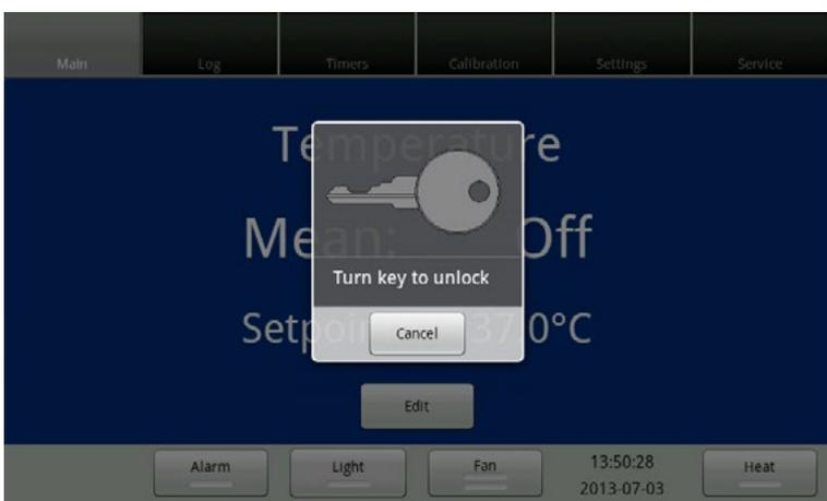
The unit cannot be switched on while it is locked. It is only possible to switch the unit on when it is unlocked and the key is in place. Turn the key on the units' side to unlock.
