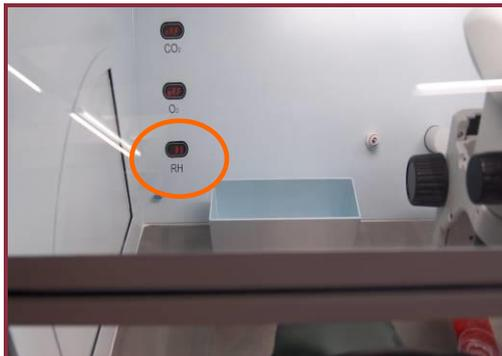
If the alarm sounds either move the reservoir to the non warmed area or remove the reservoir from the working area. If the G603 is not in use vent the working area by opening the side hatches.
