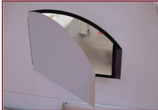
Make sure that the hatch is closed after openings. It is not spring loaded. Limit the number of openings to a minimum during procedures as it will affect the CO<sub>2</sub> and O<sub>2</sub> levels.
