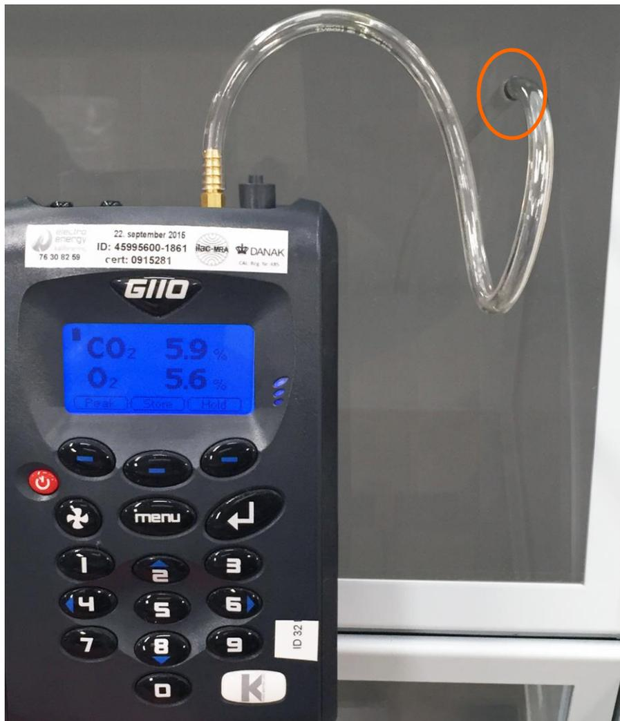
Compare the CO<sub>2</sub> readout with the value shown under 'CO2.C' in the menu and adjust if necessary.
