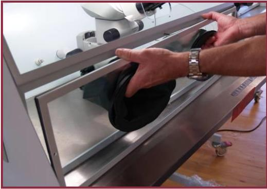
Panel removed and clear access for cleaning.
