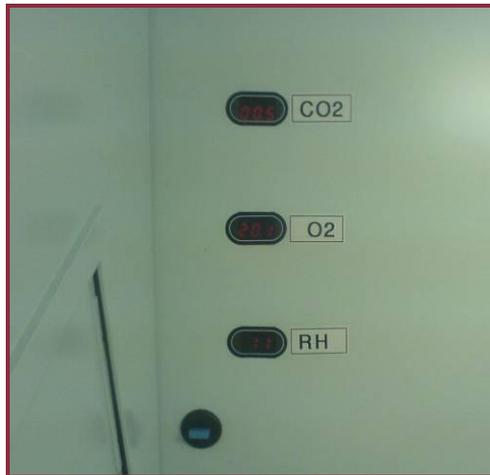
The first display from the top is used to show the status of the CO<sub>2</sub> regulator (ON or OFF) and to show the actual concentration of CO<sub>2</sub>. This display is also used to alert the user in case of any alarm that is related to the CO<sub>2</sub> regulator, wrong CO<sub>2</sub> concentration or wrong incoming gas pressure).
