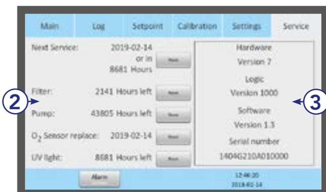
This screen (3) also displays hardware and software versions currently installed and the unit's serial number.
