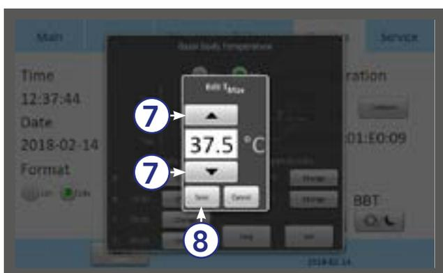
8. Adjust both the  $T_{Max}$  and the  $T_{Min}$  values by pressing the up and down arrows (7).
