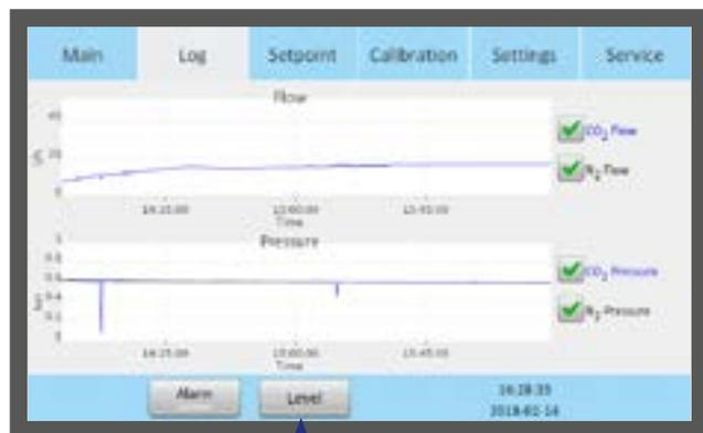
3. Press Level button (2) to return to temperature and gas concentration.
