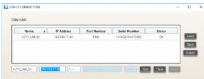
After loading a device, and performing a successful connectivity test, indicated by status "OK", logging can be started by pressing "Start".
