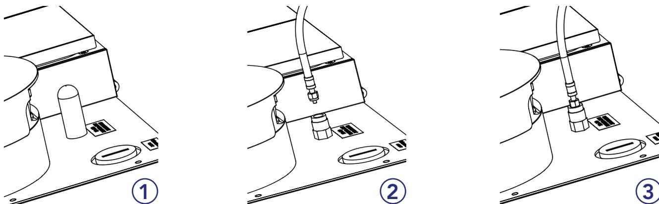
1. Connect a short length of tubing to the gas analyzer input.
