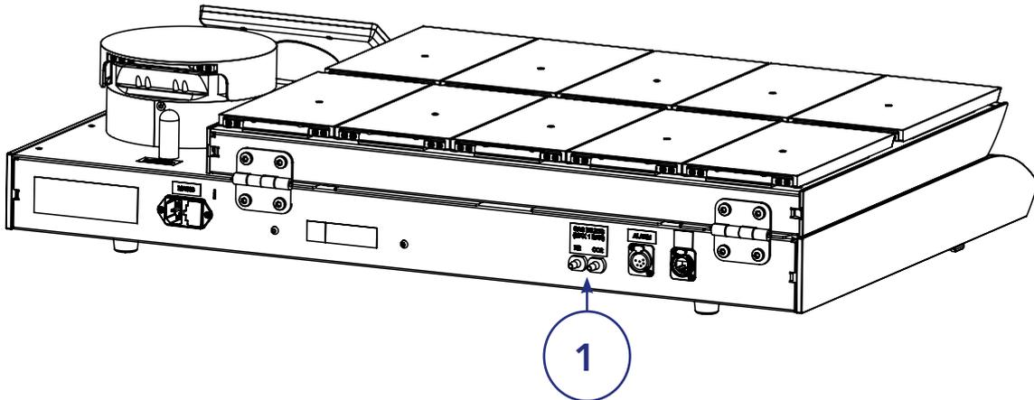
1. The G210 is not supplied sterile and should be cleaned before use. Make sure the gas input and output ports at the back of the incubator are also cleaned. See "Section 12 - Maintenance" on page 40.
