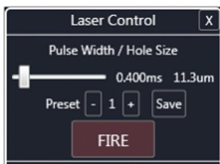
Choose the preset by clicking the + or - buttons. To change a preset, select the preset, set the desired value using the slider, and click the **Save** button.
