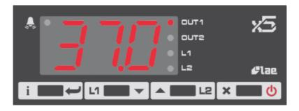
Thee display shows the temperature readout from the chosen channel (only channel 1 is used on this application). In case of an alarm situation a red light will start flashing in the top left-hand corner of the display. On the right-hand side of the display it is indicated which parameter is shown in the display. Below is listed all possible values and messages that can be shown in the display:
