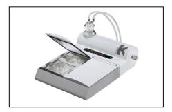
Note Always place a warming block in the chambers during warm up and be careful with the heated area under the humidifier bottle as it will become hot.
