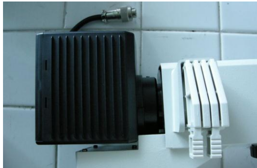
50W lamphouse mounted to the diascopic 100W illumination pillar
