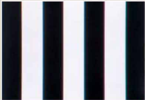
Image where chromatic aberration has been corrected in the SMZ1500
