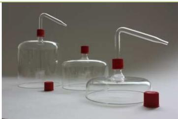
6. Use a glass hood (option, not provided as standard) and connect the elbow with a silicon tube and connect the other end of the silicon tube to the outlet of the gas located next to the humidifier glass bottle.
