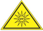
**For protection against unintended UV radiation which will harm eyes and skin, use the timer to start the UV decontamination when no personnel is present in the room where the workstation is located.**
