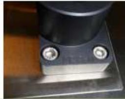
15. Place pole (L300 = WG0400 or L400= WG0359) into mounting block. Secure with M4x8 grub screw (WG0816) at the back.
