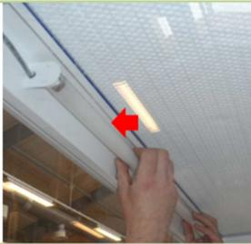
Two light tubes are installed in a MARS Workstation between the laminator air panel and the HEPA filter.
