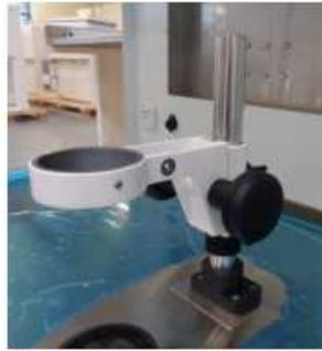
10. Place microscope on to supporting bracket.
